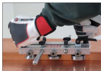
Scorre in avanti tramite le maniglie superiori. Forward move by upper handholds.
